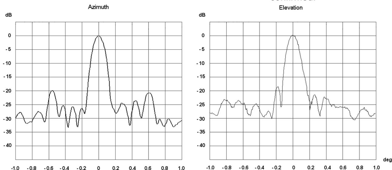
There was a significant improvement of the pattern and about 0.4 dB rise of the antenna gain. It was hard to say whether it's high or low rise. To evaluate the effectiveness of the lens one need to know the scale of the problem. We need to know the difference in gain of my non-ideal antenna and the antenna with an ideal shape of the reflector.
