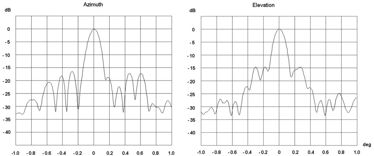
Nevertheless, I quickly calculated the lens and produced it from three 1mm Teflon layers. There was a significant improvement. The level of the first side lobe was reduced by 6 ... 7 dB. Unfortunately it was no noticeable increase in antenna gain. So I decided not to use the lens in future EME tests.
