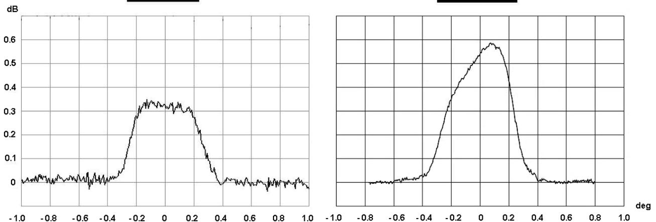
Moon noise on 77 GHz is strongly depends on the phase of the Moon. The noise level of the full Moon is about two times higher than of the new Moon. In contrast to the lower frequency bands, you cannot find the center of the moon by the noise maximum, and need to be guided by the edge of the lunar disk.
