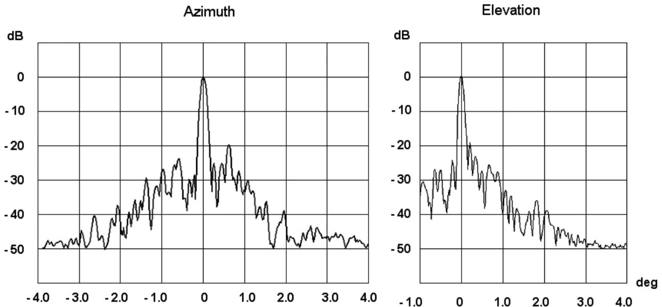
So, we have the data to analyze a part of the radiation pattern, adjacent to the main lobe. From the most common considerations it is clear that smooth deviations from the ideal shape of the dish affecting only this part of the pattern. Based on these diagrams the three-dimensional pattern of the antenna was built for two cases - with and without the lens. The integration of 3D pattern gives the following results.
