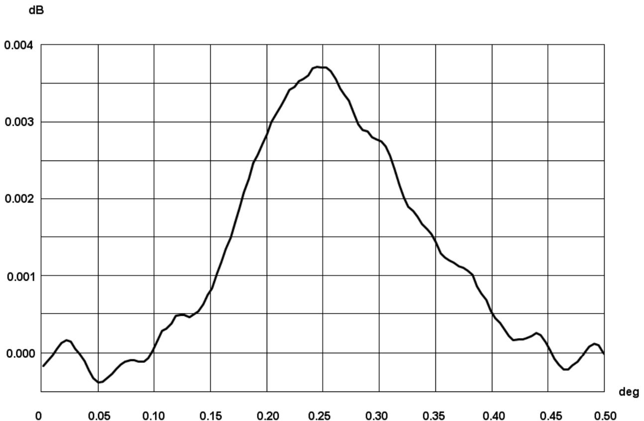
You can see the result of 10 recordings averaging. I have no reliable explanation for this effect. It seems that much depends on the state of the atmosphere. On February 1 the temperature rose and the state of the atmosphere obviously changed compared with previous frosty nights. Perhaps the atmosphere became quieter and it reduced the signal fluctuations. In any case I plan to do it again next winter to understand the problem.
