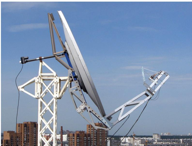
The first measurements showed that the radiation pattern is far from perfect, especially in the elevation plane.
